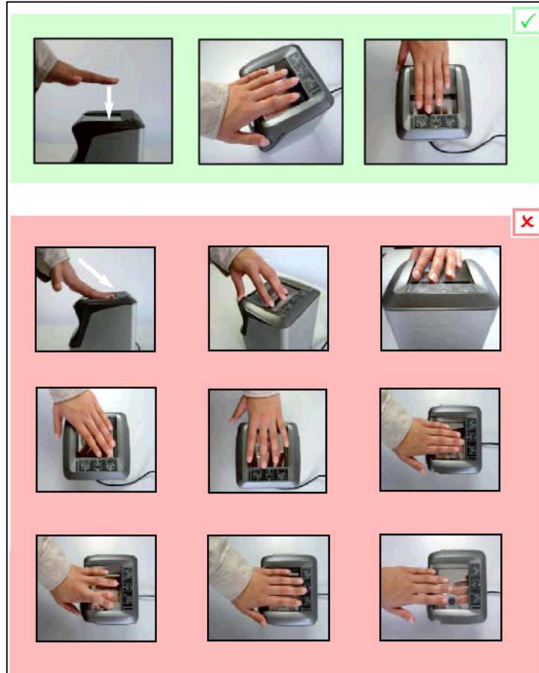
Figure 28: Correct way of placing fingers on the fingerprint scanner platen
